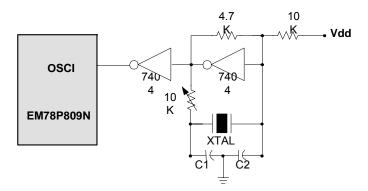
Fig. 33. Crystal/Resonator-Parallel Mode Circuit
